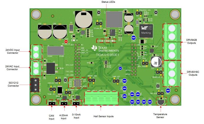
Figure 3-1. TIDA-010950 PCB Connections
