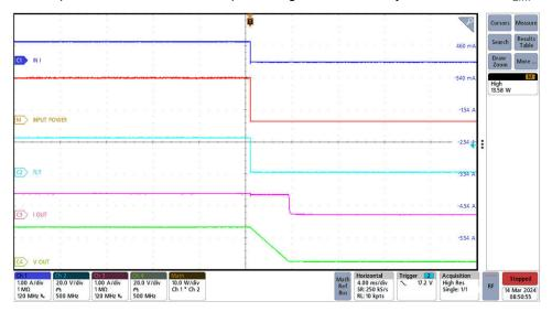
Figure 3-7. E-Fuse Power Limiting
