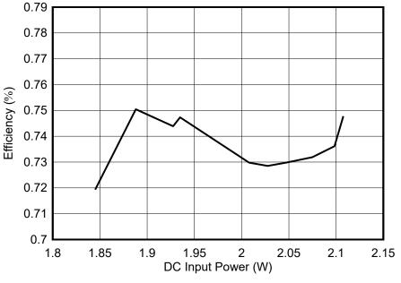
Figure 3-24. DRV8428 Efficiency Over Input Power
