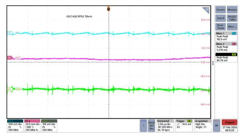
Figure 3-12. TPS62932 Ripple at 750mA Load
