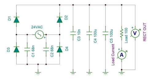
Figure 2-3. 24VAC Rectification TINA-TI Simulation Circuit
