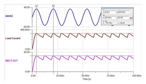
Figure 2-4. 24VAC Rectification TINA-TI Simulation Waveforms
