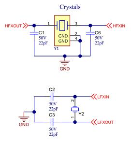
Figure 2-12. External Crystal Oscillators for TCAN Communication
