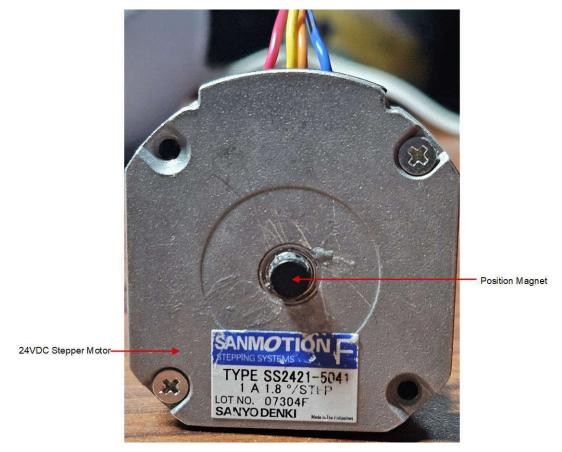
Figure 3-21. Stepper Motor Setup with Position Magnet
