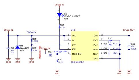
Figure 2-5. TPS16410 E-Fuse Circuit Implementation
