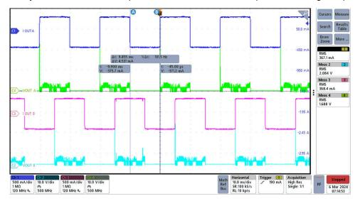
Figure 3-23. DRV8428 Output Current and Voltage with Smart Tune Ripple Control
