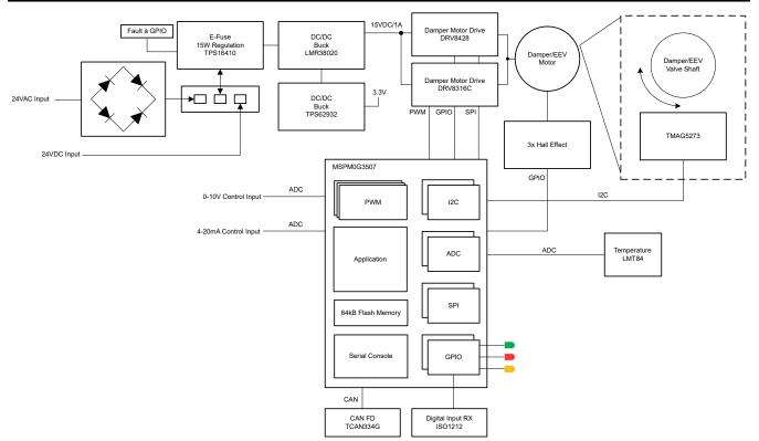
Figure 2-1. System Block Diagram
