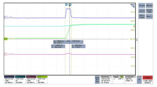
Figure 3-5. E-Fuse Start-up at No Load
