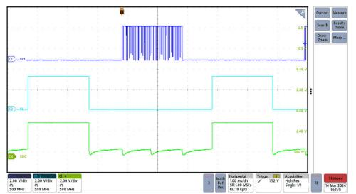
Figure 3-19. DRV8316C INH, INL, and SOx During Motor Operation (OTL)
