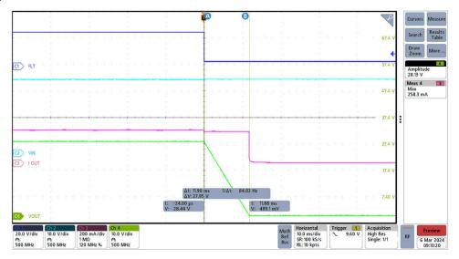
Figure 3-8. E-Fuse Input Overvoltage Protection Response
