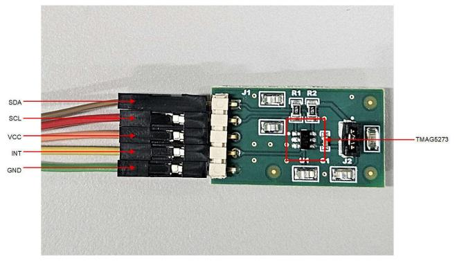
Figure 3-15. TMAG5273 Remote Sensing Board for BLDC Motor Position Sensing
