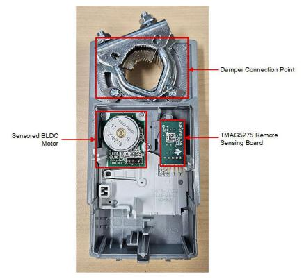
Figure 3-14. BLDC Damper Control Test Setup
