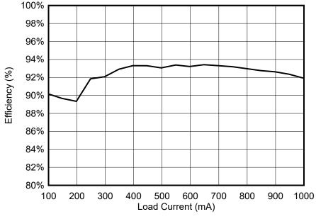
Figure 3-11. LMR38020 Efficiency Over Load With 24VAC Input
