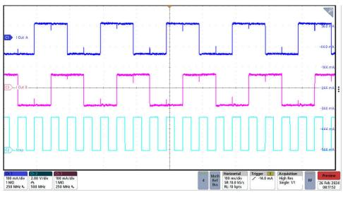
Figure 3-22. DRV8428 Phase Output and STEP Control Signal
