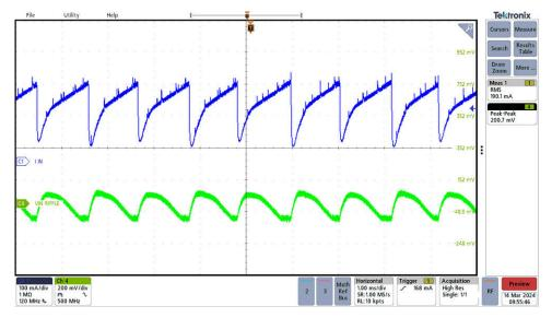
Figure 3-18. DRV8316C Input Current and Input Voltage Ripple During Operation
