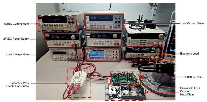
Figure 3-2. Lab Bench Test Setup I
