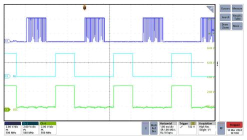
Figure 3-20. DRV8316C INH, INL, and SOx During Motor Operation (OTR)
