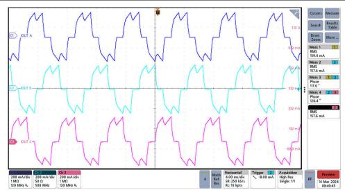
Figure 3-17. DRV8316C Output Current During Motor Operation
