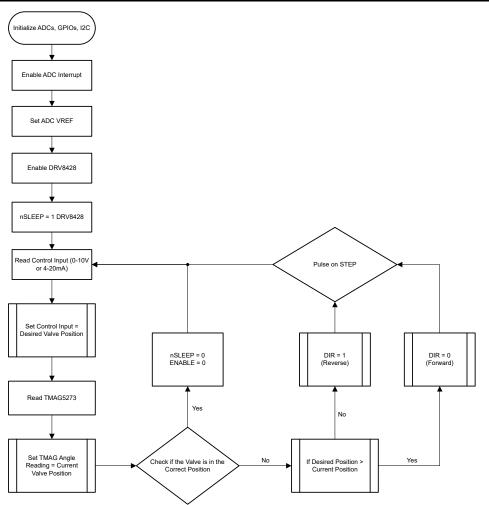
Figure 2-16. Stepper Motor Control Software Control Loop Diagram (Control Input Based)
