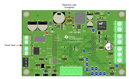
Figure 3-4. Board Connections Used to Test the TPS16410 E-Fuse
