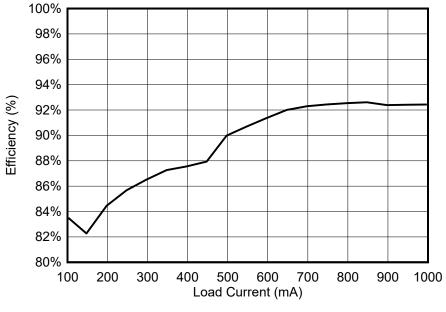
Figure 3-13. TPS62932 Efficiency Over Load
