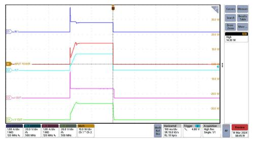
Figure 3-6. E-Fuse Regulation During Voltage Turn-On at High Load
