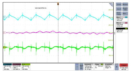
Figure 3-9. LMR38020 Output Voltage Ripple at 1A Load
