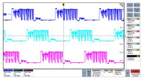
Figure 3-16. DRV8316C Voltage Output for Each Phase
