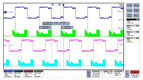
Figure 3-25. DRV8428 Output Current and Voltage With Smart Tune Dynamic Decay
