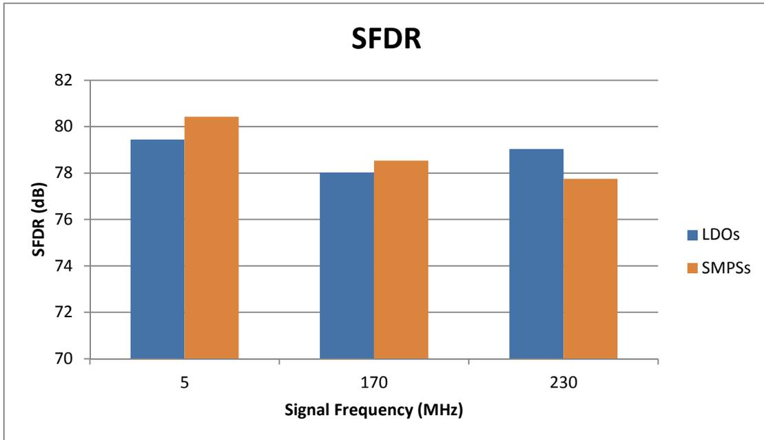
**Figure 3. SFDR comparison of the LDO power solution to the SMPS power solution**
