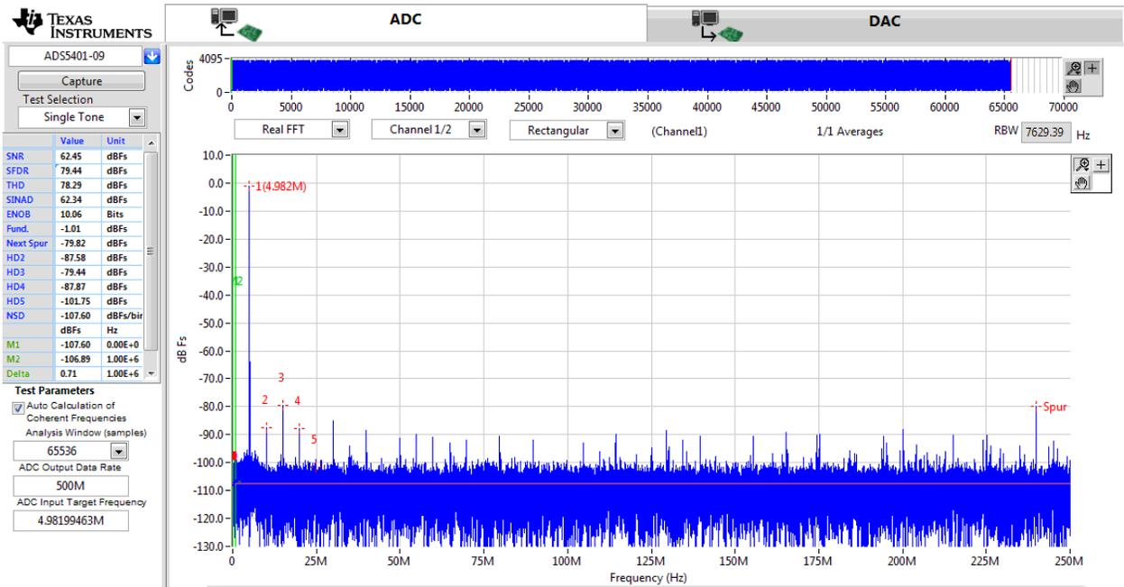
**Figure A-1. ADS5407 powered with LDOs and 5-MHz signal frequency**
