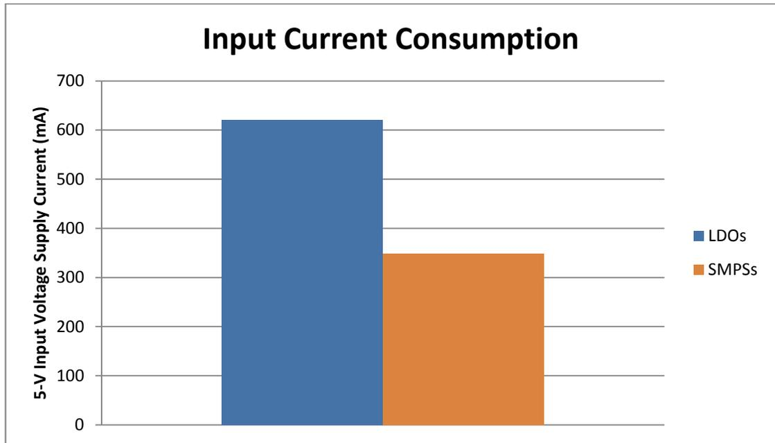
**Figure 4. Input current consumption comparison of the LDO power solution to the SMPS power solution**
