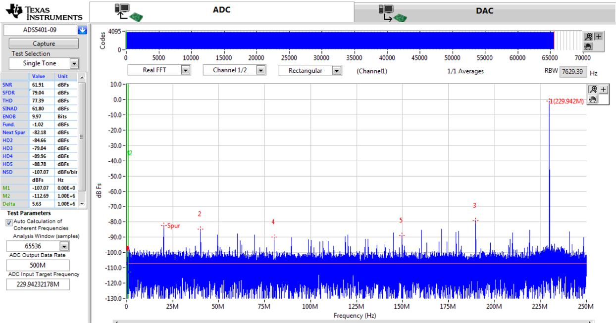
**Figure A-5. ADS5407 powered with LDOs and 230-MHz signal frequency**
