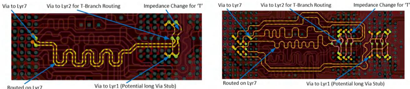
**Figure 3-7. Example LPDDR4 Clock and CA Routing**
