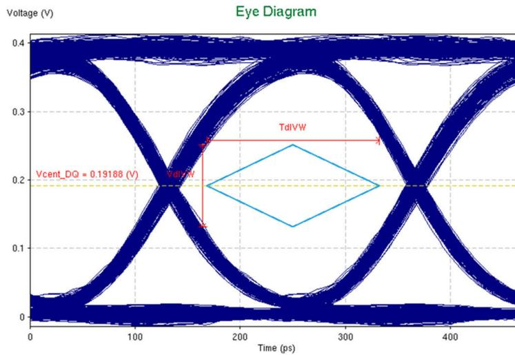
Figure 3-4. Example Simulated LPDDR4-4266 Read Eye With Diamond-Shaped Eye Mask
