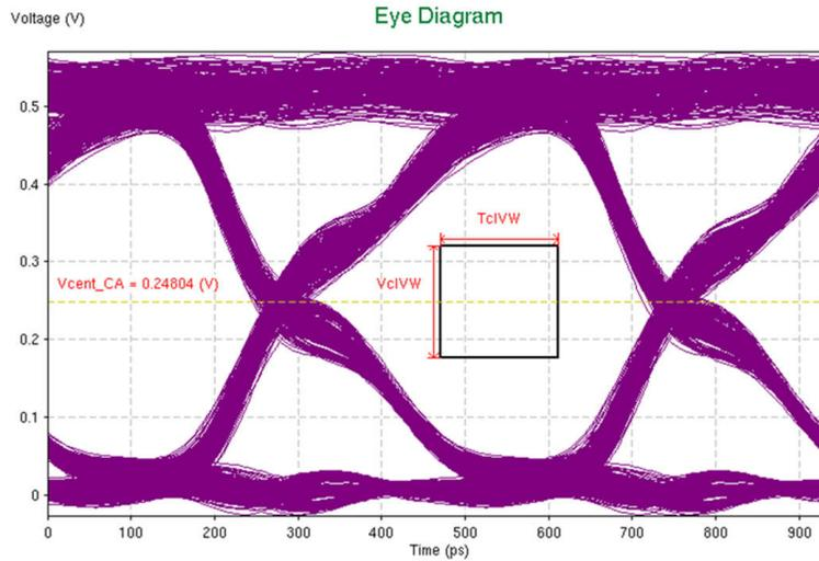
Figure 3-6. Example Simulated LPDDR4-4266 CA Eye With Rectangular JEDEC Eye Mask
