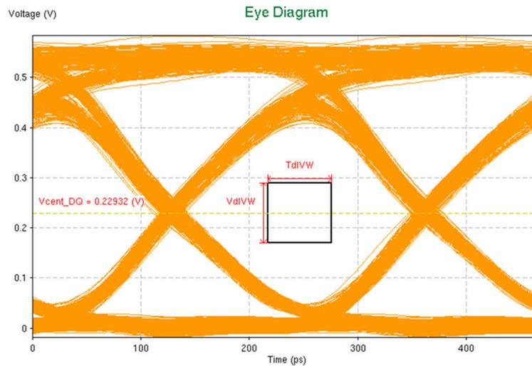
Figure 3-5. Example Simulated LPDDR4-4266 Write Eye With Rectangular JEDEC Eye Mask
