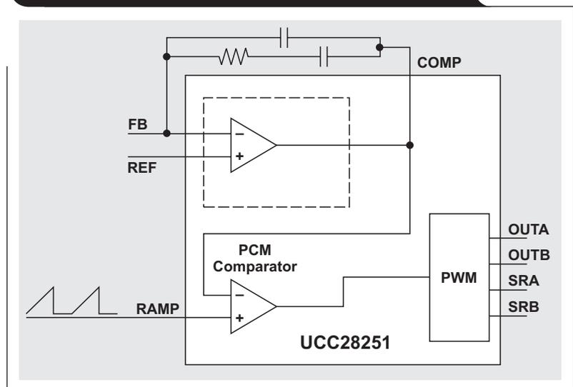
Compared with a primary analog controller solution, it becomes more difficult for the digital controller to quickly and accurately detect the input voltage transients occurring on the transformer's primary side. In a purely digital solution, the designer must consider further complexities such as A/D conversion delay, digital processing delay, and digital pulse-width modulator (DPWM) generating delay.
