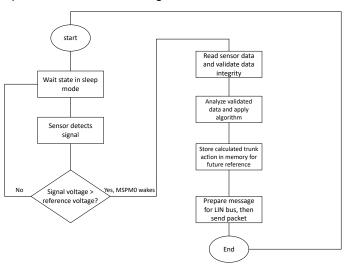
Figure 7. MSPM0 Kick to-open-Trunk Module Example Flow Chart
