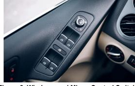
Figure 2. Windows and Mirror Control Switches
