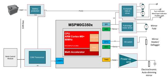
Figure 5. Side Mirror Module System Block Diagram
