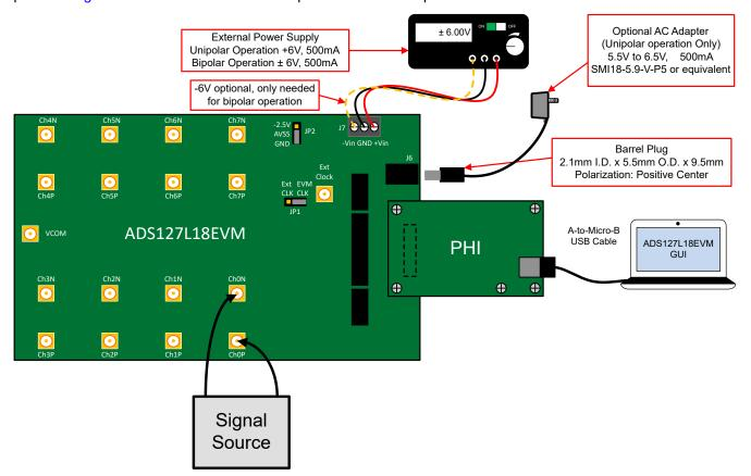
Figure 2-2. Power Connections
