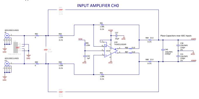
Figure 2-4. ADC Input Amplifier
