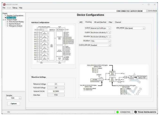
Figure 4-6. Clocking Configuration
