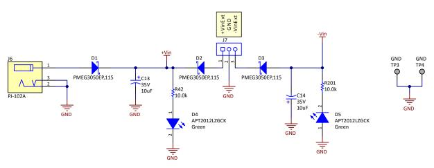
Figure 2-11. External Power Supply Connections
