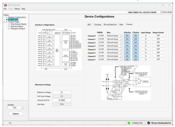
Figure 4-9. Channel Configuration
