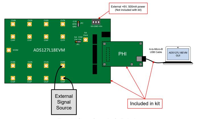
Figure 1-1. System Connection for Evaluation
