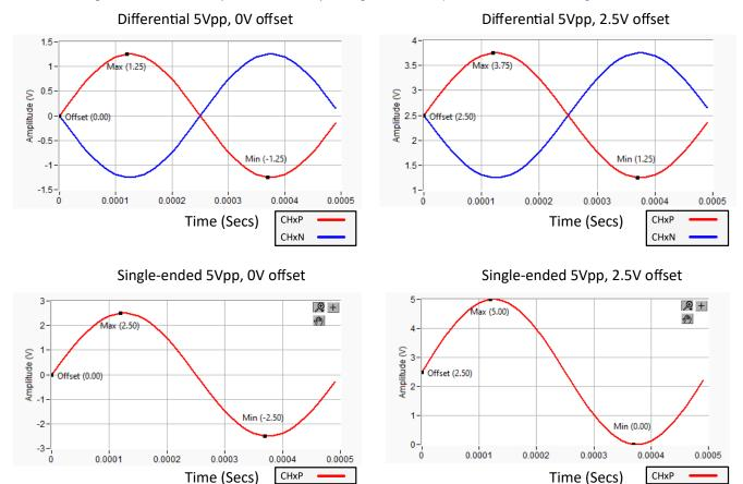
Figure 2-1. Maximum input signal range (Vref = 2.5V)
