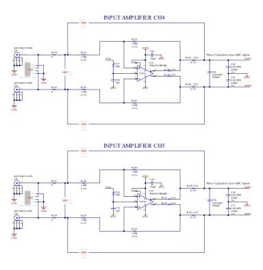
Figure 5-6. ADS127L18EVM Input Channels 4 and 5 Schematic
