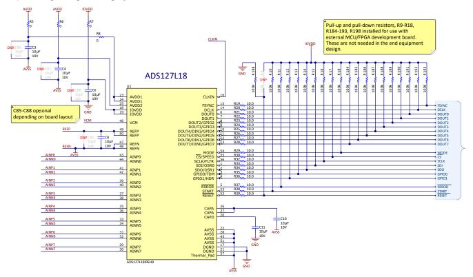
Figure 2-3. ADS127L18 Connections and Decoupling
