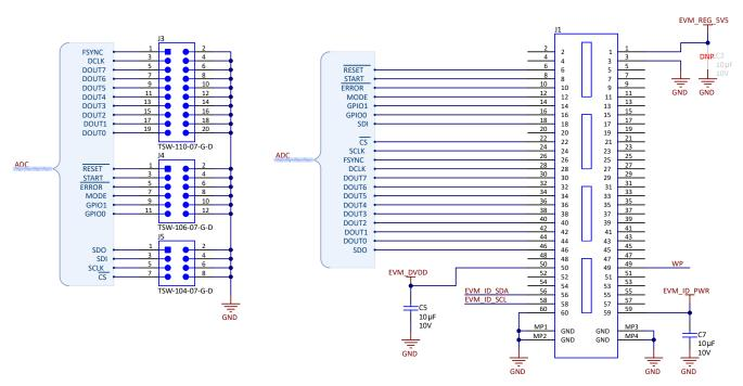
Figure 2-9. Connections to Digital Signals on PHI and Test Points
