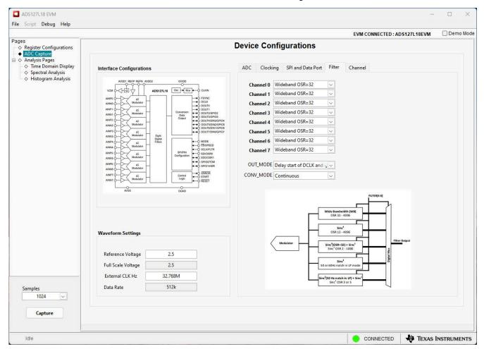
Figure 4-8. Filter Configuration
