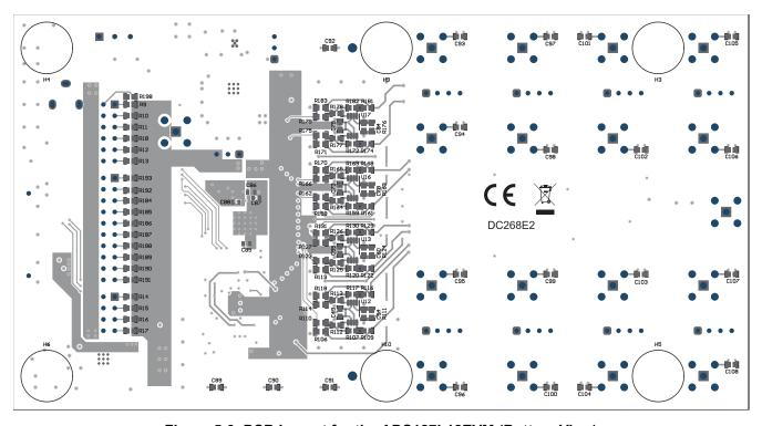
Figure 5-9. PCB Layout for the ADS127L18EVM (Bottom View)
